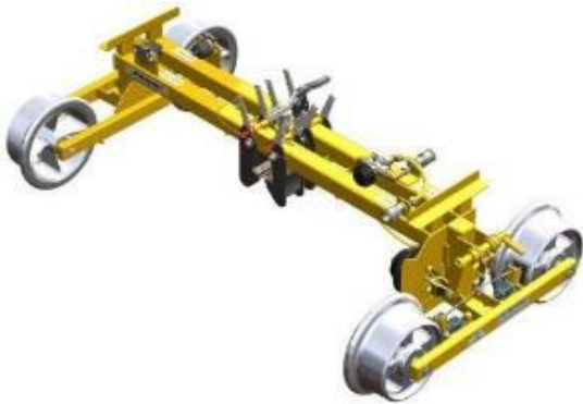
LRT 2nd trailer (Bogie)
